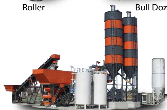
Concrete Batching Plant
