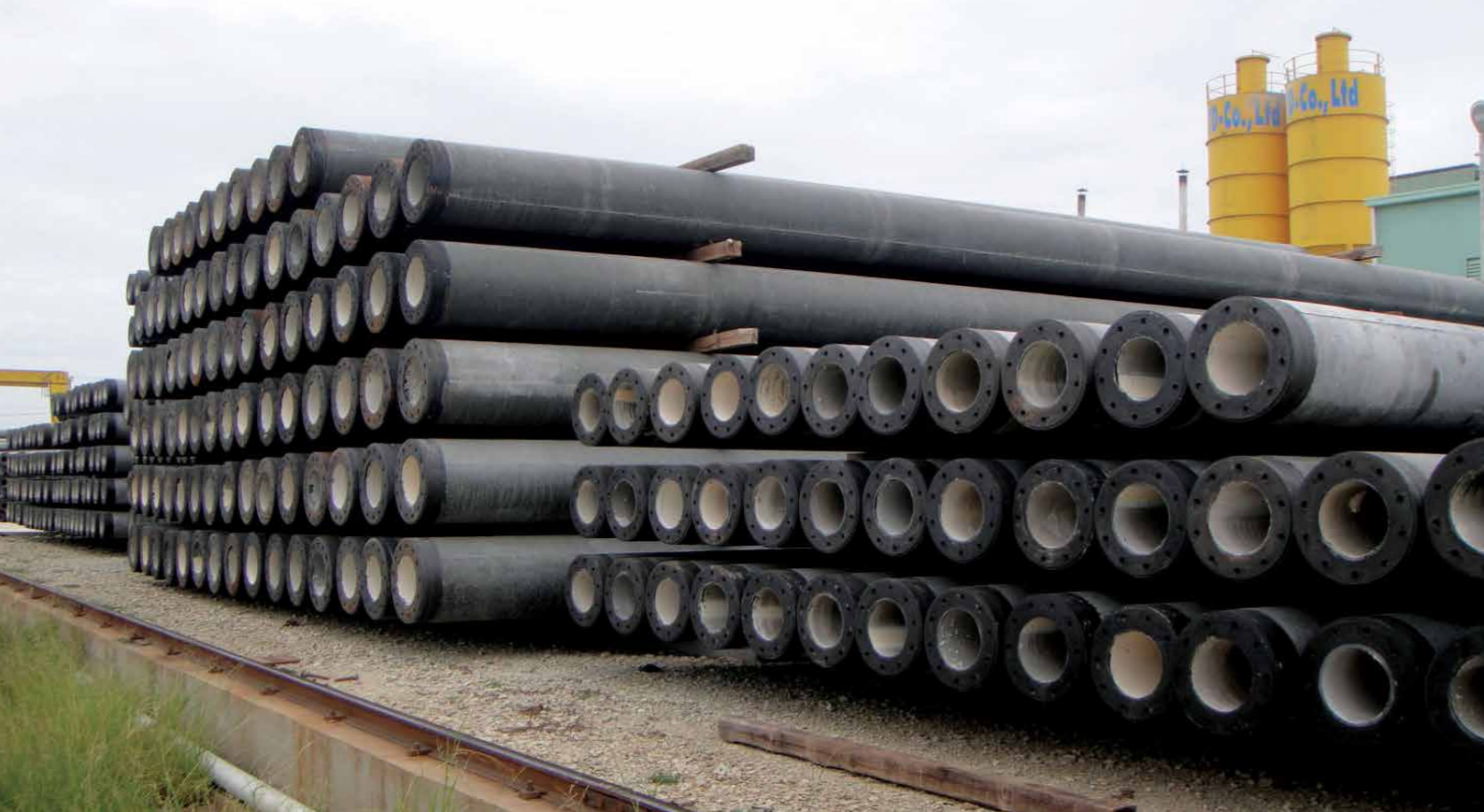
📍 Pile yard at 7FTD's precast concrete site
