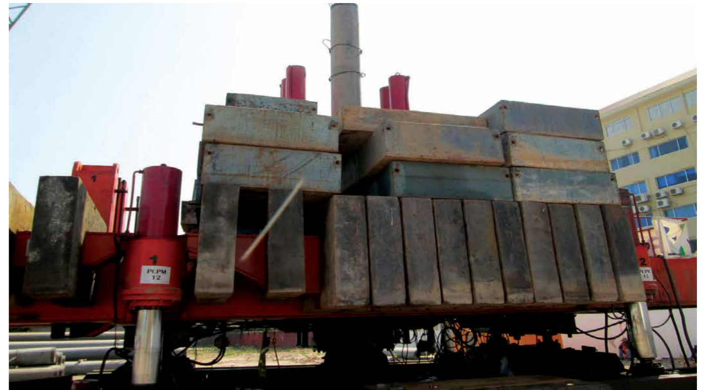
Hydraulic injection pile
