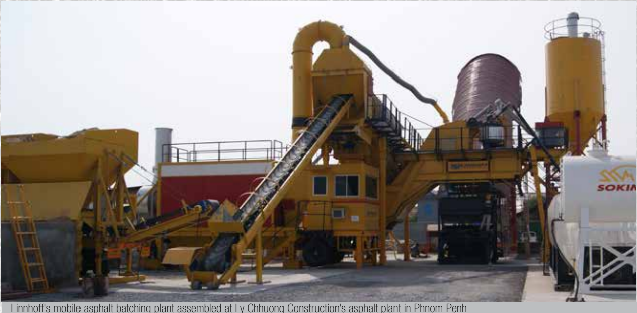
Linnhoff's mobile asphalt batching plant assembled at Ly Chhuong Construction's asphalt plant in Phnom Penh
