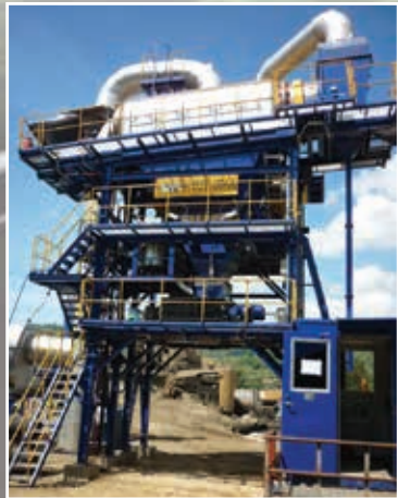
CMX1500 in Philippines (CompactMix Asphalt Mixing Plant, 90 - 100 TPH @5% Moisture)
