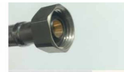
Plastic nipple looks as a brass one, but its weight gives us know what it's really made of.
