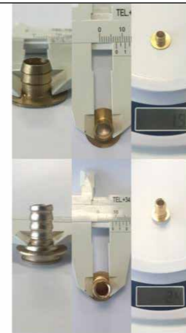
Plastic nipple looks as a brass one, but its weight gives us know what it's really made of.
