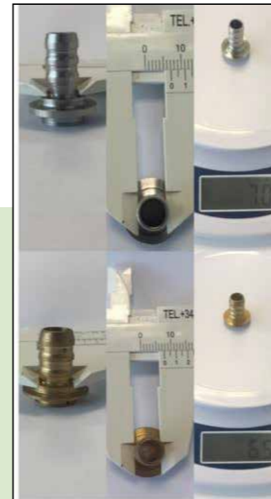
Brass and stainless steel good quality nipples.
