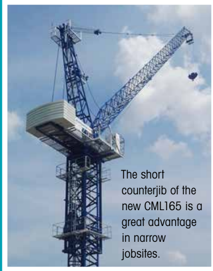
Comansa CM's new luffer has a maximum lifting capacity of 12 tonnes.
